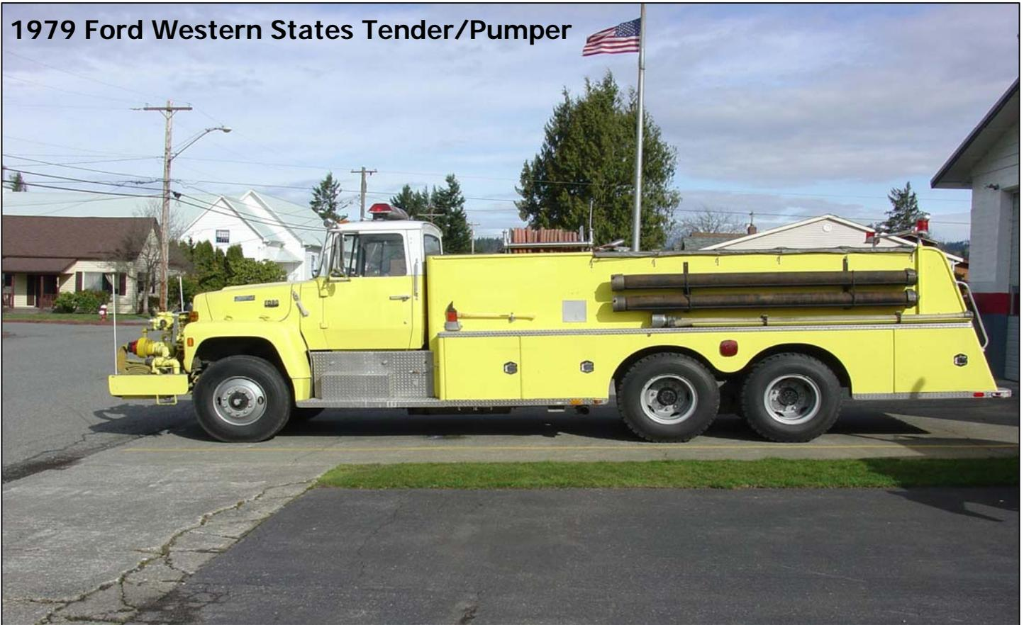
**Chassis:** Ford L9000, Detroit Diesel 8v71N 330hp, Eaton Fuller 10 Speed Manual Transmission 13,292 Miles, 531 Hours
